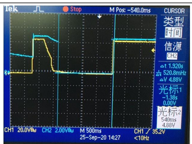
Output response & load (5V / 1.2A)
